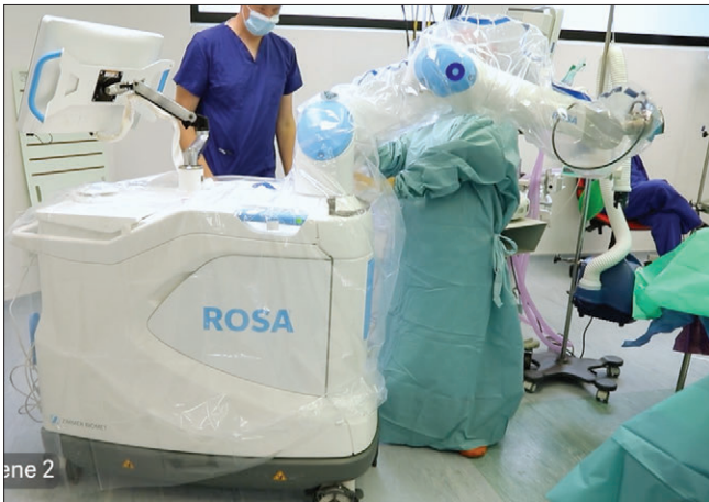
Figure 8: Robot- ROSA used for RAS in total knee arthroplasty. RAS: Robotic-assisted surgery
