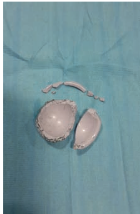
Fig. 3. Fractured ceramic liner.
