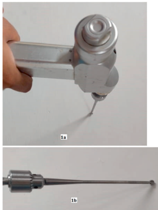
Fig. 1. Perpendicular drilling of wall (1a) and oblique drilling of wall (1b) - appreciate the change in intended aperture shape-circular with perpendicular drilling and elliptical with oblique drilling.
