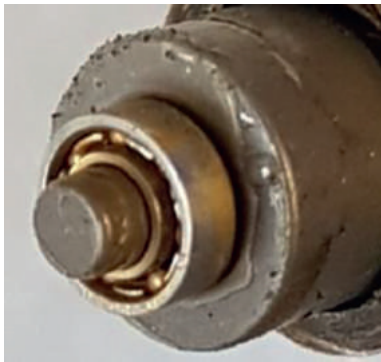
Fig. E1. Radial bearing on magnet shaft.
