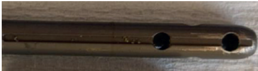
Fig. E7. Extending bar showing debris and longitudinal surface damage.
