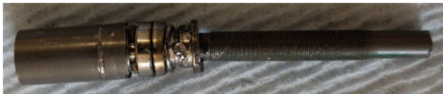
Fig. C3. Component sub-assembly from nail N001 post-cutting.
