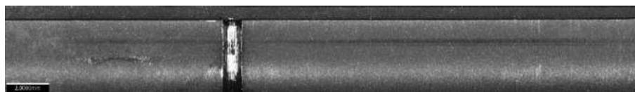
Fig. 7. Alicona image of extending bar longitudinal damage. Both fretting and pitting corrosion are present on this view.
