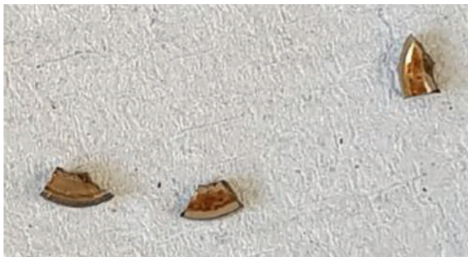
Fig. E2. Axial bearing race, fractured into three pieces, showing discolored raceway.
